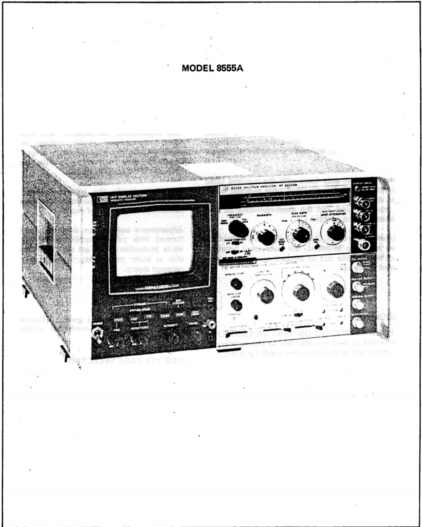
Figure 1-1. Model 8555A Spectrum Analyzer RF Section with 8552B IF Section and 141T Display Section
